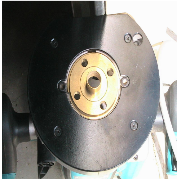
Correct Makita sub-base with 25mm OD metal template guide bush installed.
