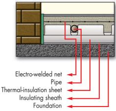
The same application can be created by using sheets provided with protective layer, 5cm pass, green- and black-coloured.
