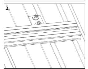
**3. Placing second strut on roof (do not fasten down yet):** Following the previous steps, place the second strut at the desired location. so that the bolt slots within the two GRIPPERFIX Struts are the same distance apart and consistent with the distance between mounting locations on the base of the object being mounted. **(Fig. 3). DO NOT fasten to roof at this point.**
