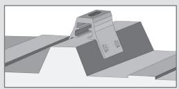
All pre-punched holes must be used to achieve tested strength. Fasteners included.
